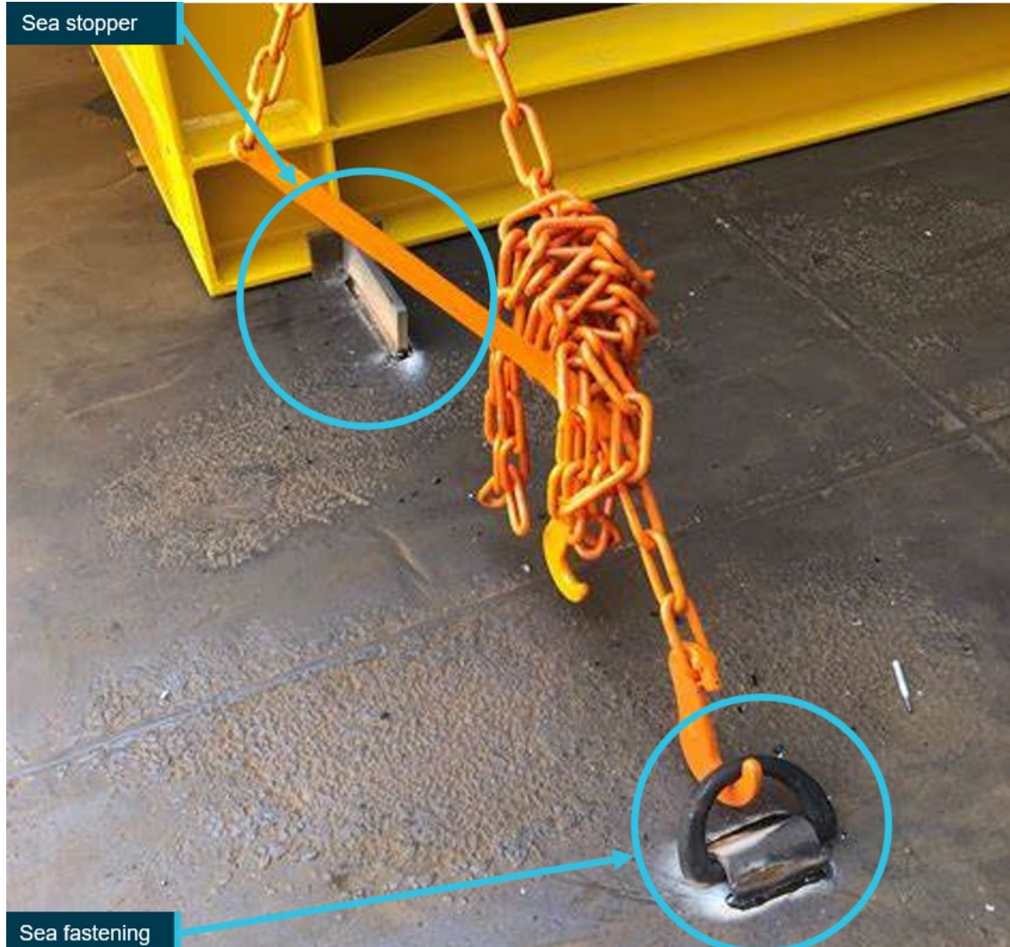
Figure 6: Example of project cargo securing
