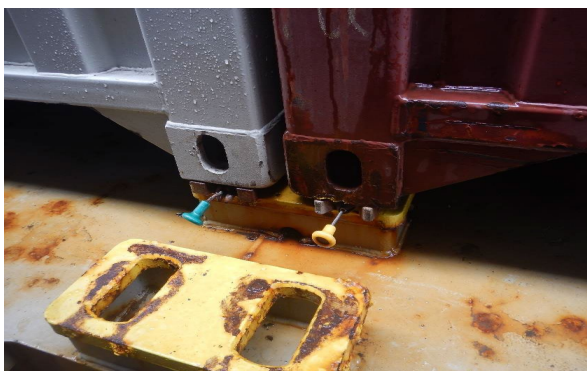
Mixed locks at base of stack
