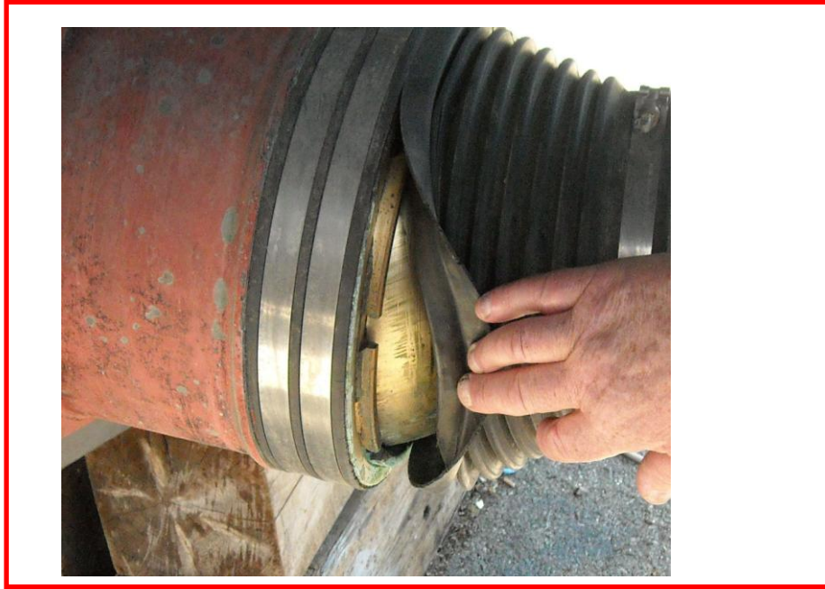
Photograph 8 A Torn rubber Glove on a Surface Piecing Propeller Pantograph
