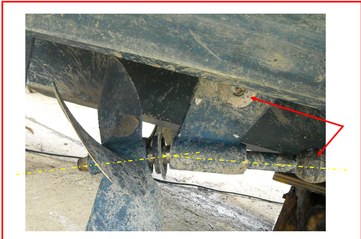
Photograph 7 A Bent Propeller Shaft
