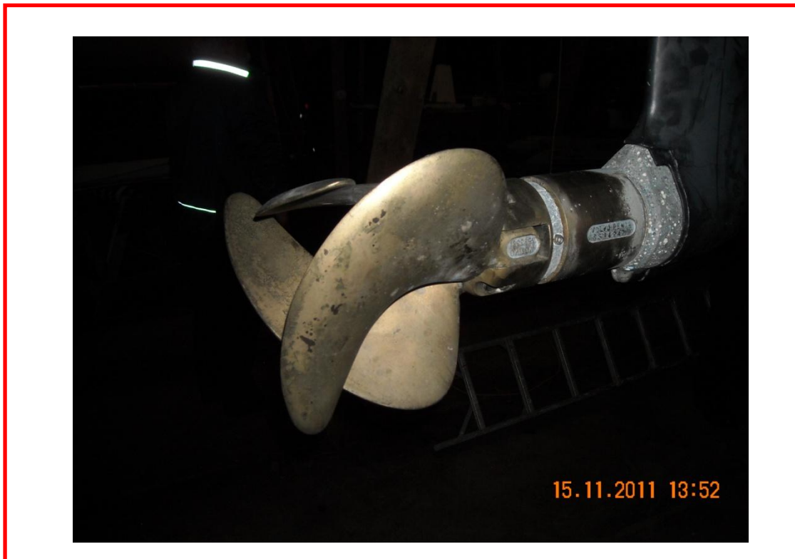
Photograph 2 Folding Propeller in Closed Mode
