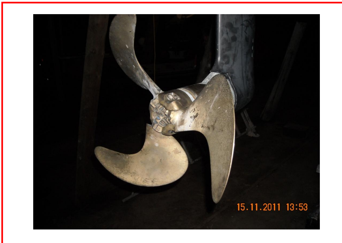
Photograph 1 Folding Propeller in Open Mode
