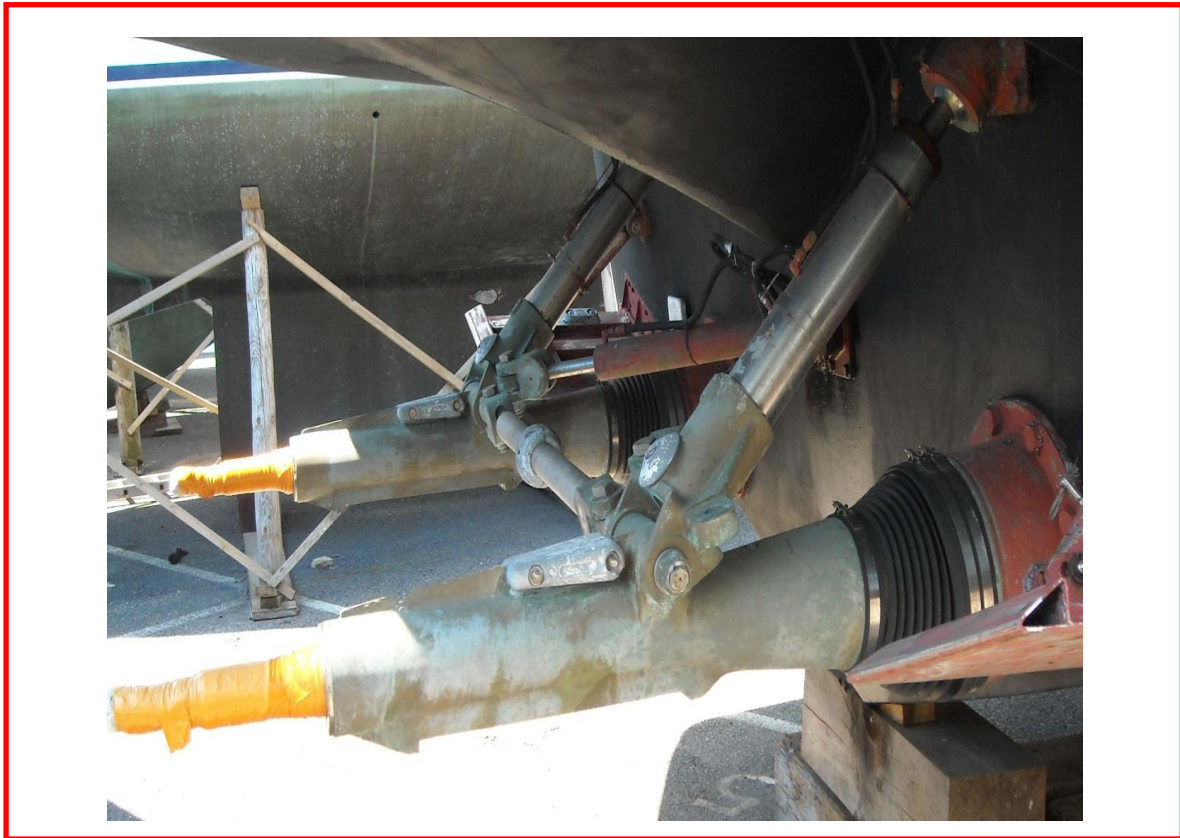
Photograph 4 Pantograph Arrangement on a Surface Piercing Propeller
